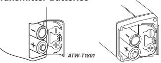
Battery Selection Each transmitter uses two 1.5V AA batteries, not included. Alkaline type is recommended. Always replace both batteries. Make certain the transmitter power is Off before replacing batteries.
